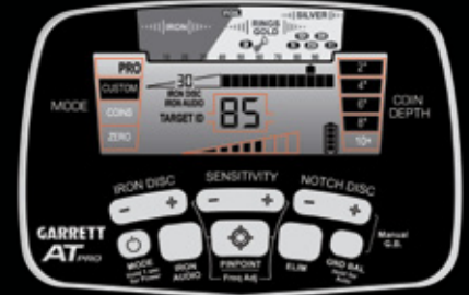
AT Pro control panel
